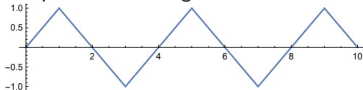
$$= \frac{8}{\pi^2} \left[ \sin(2\pi t/4) - \dots \right. \\ \left. - \frac{1}{9} \sin(6\pi t/4) + \dots \right. \\ \left. + \frac{1}{25} \sin(10\pi t/4) \pm \dots \right]$$
